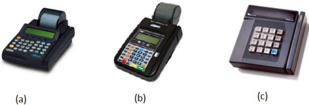
Figure 1: Dial-Up terminals. (a) Verifone, the first modern card swiping machine. (b) Hypercom, the main competitor of Verifone. (c) Lipman, the wireless processing terminal, but having the same bulky form factor.
