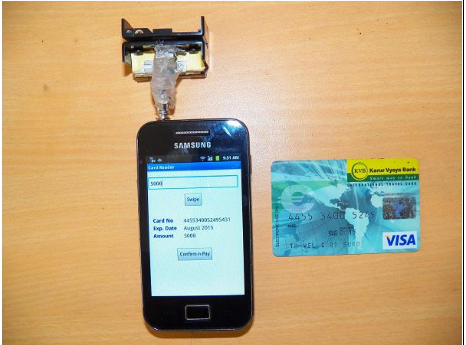
Figure 14: A VISA debit card along with the read data shown by the app
