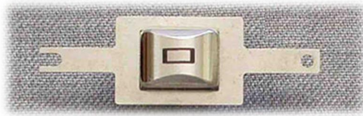
Figure 7: Read head for reading the magnetic stripe card.
