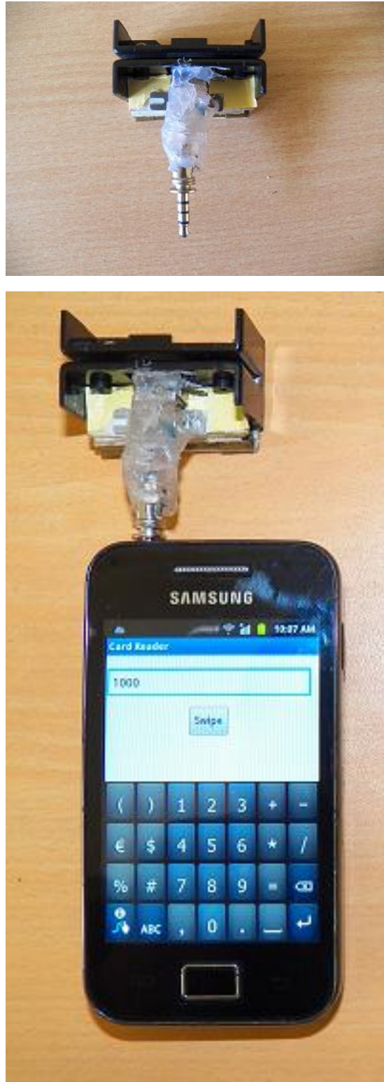
Figure 12: (Top) The analog card reader made for this study. (Bottom) The card reader plugged into the mobile phone
